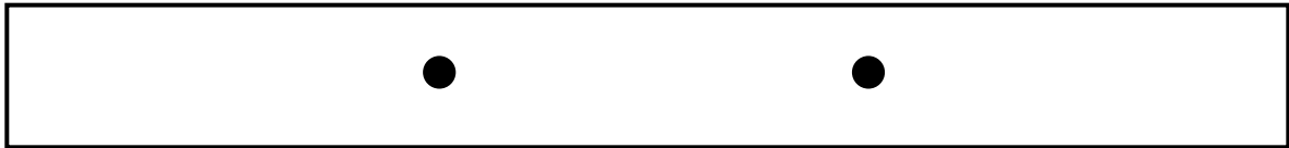
Example 1: Two 1/8 in. (3.2 mm) discontinuities
