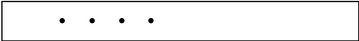
Example 4: Four 1/16 in. (1.6 mm) discontinuities
